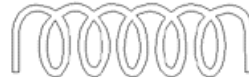
Figure 2-7. Circuit symbol for an ideal (loss-less) inductor. An ideal inductor is linear and time-invariant.
